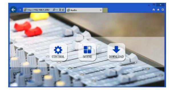
Control: Control channel parameters and enable and disable each processor
