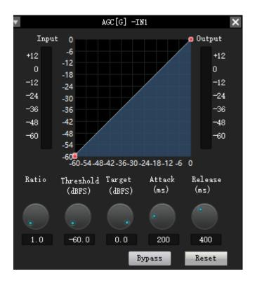
The purpose of automatic gain control is to achieve the target level of signals with uncertain levels while maintaining the dynamic range of the volume.
