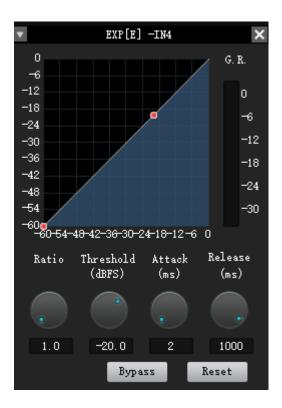
The Expander is a dynamic range of input that increases according to the user's requirements.
