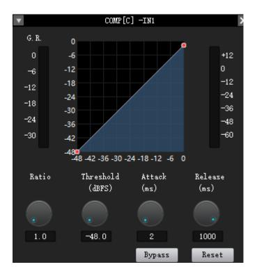
The compressor is used to reduce the dynamic range of the signal above a user-defined threshold. The signal level below the threshold remains unchanged.
